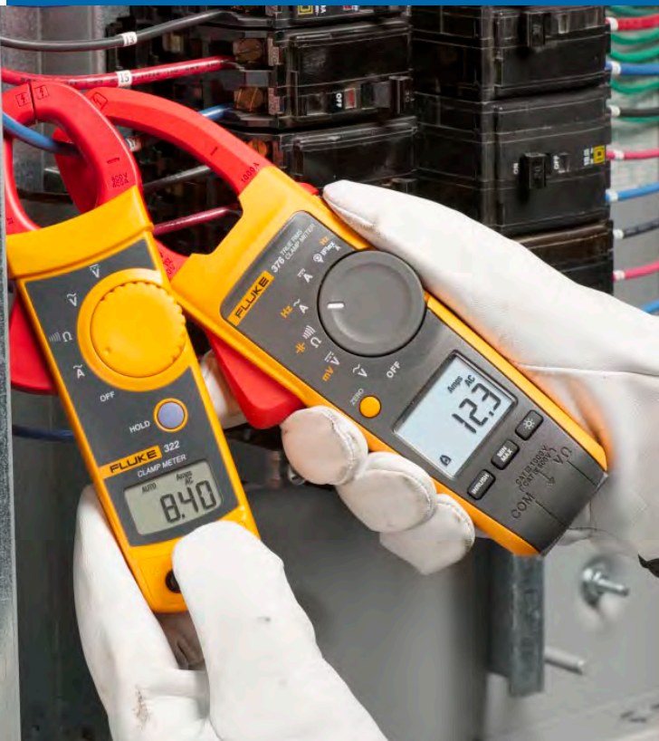
One current—two readings. Which do you trust? The branch circuit above feeds a non-linear load with distorted current. The true-rms clamp reads correctly but the average responding clamp reads low by 32 percent.
