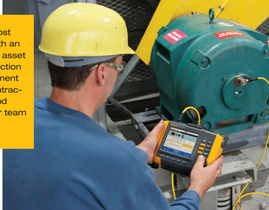
The 810 Vibration Tester monitors an operational motor.
