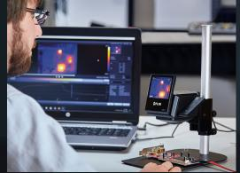
Connect over USB a computer to analyze data in FLIR Tools+
