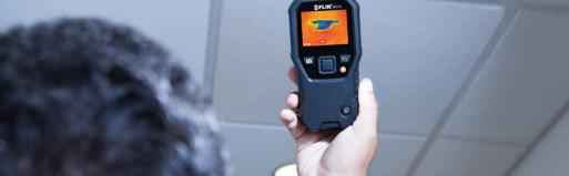
Featuring IGM technology powered by a built-in thermal imaging sensor, the MR176 and MR160 can visually guide you to the precise spot that moisture may be hiding
