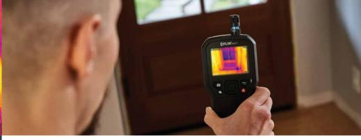
Combining the advantages of a high-resolution infrared imaging sensor, FLIR MSX® image technology, and a laser pointer, the all-in-one MR277 building inspection system helps you quickly locate, clearly identify, and easily document critical moisture and building envelope issues.
