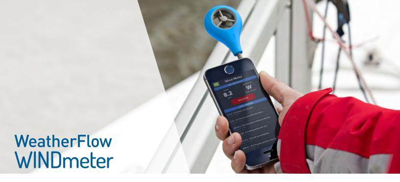
The WeatherFlow Wind Meter is a pocket-sized anemometer that captures highly accurate wind measurements. It connects to your iOS or Android device via the audio jack. Use the free 'Wind Meter' app or other compatible apps to record and share wind reports.
