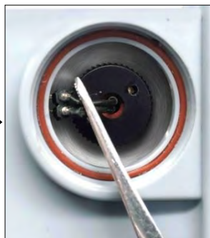
Use a tweezer to unplug the socket
