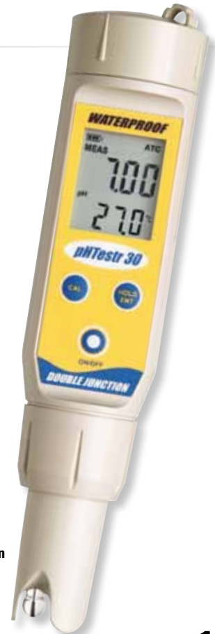
35634-30 Waterproof double-junction pHTestr 30
