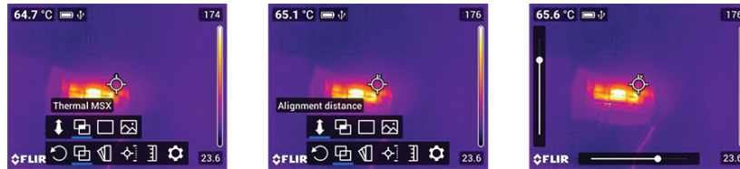
Figure 7.5 Select the Thermal MSX mode and then the Alignment Distance option. Use the sliders (left side and bottom of the display) to align the Digital Camera image with the Thermal image. Use the left/right and up/down arrow buttons to make the adjustments.
