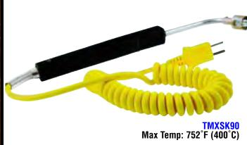
The TMXSK90 is the fastest and most accurate handheld K-type surface probe providing accurate readings in less than 5 seconds. The sensor is made from flat-spring ribbons of thermocouple material for contact on uneven surfaces. An angled head for measuring hard to reach surfaces and a 3 foot coiled lead for durability and long reach. The exposed junction provides for fast response and is compatible with any other instrument with a K-Type input.
