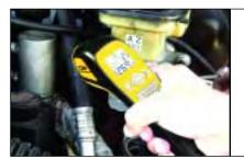
The unit offers simple one-handed operation, laser point sighting, a backlit display, °C/°F select ability and an automatic power off feature.
