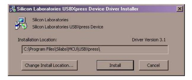
To install the driver manually, plug the VBDL100 into an available USB port on the PC. If this is the first time that the VBDL100 is connected to the particular port on the PC, the
