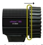
The Clear Borofloat Filter will remain inside the protector. To remove the Clear Borofloat Filter (130089), peel around the edge of the rubber cover/filter holder and push the filter out. To replace or reinsert the Clear Borofloat Filter into the rubber cover/filter holder, slide the Clear Borofloat Filter into the channel of the rubber cover/filter holder. Manipulate the rubber cover around the filter. Assure the filter is evenly seated.
