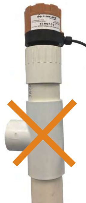
Avoid the use of a tee within the stand pipe. A tee can create false signals impeding the sensor's performance.
