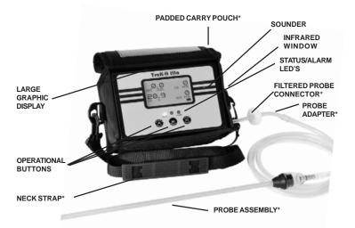
**TRAK-IT®IIIa** instruments are constructed of durable stainless steel to withstand the rigors of field use.
