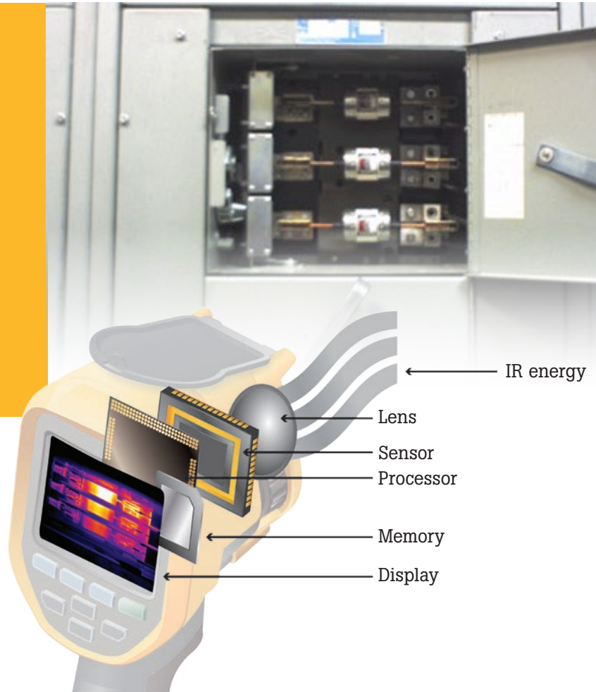
Figure 1. Anatomy of an infrared camera
