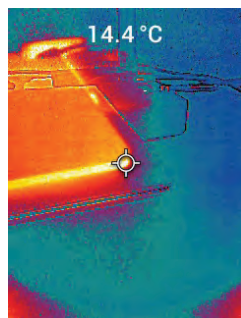
Figure 5.1 Combined Thermal and Visible Image (MSX®)
