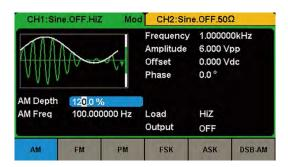
The T3AFG range of Function/Arbitrary Waveform Generators support a wide range of modulation types including AM, FM, PM, FSK, ASK, PSK and DSB-AM.
