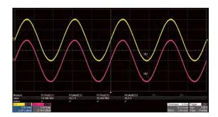
Output amplitude into a high impedance load can be as high 20 Vpp at frequencies up to 20 MHz, and 10 Vpp for fraguencies greater than 20 MUZ
