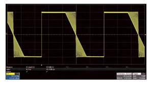
The rise/fall times can be set independently to a minimum of 8.4 ns at any frequency and to a maximum of 22.4s.
