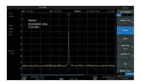
Sine wave output exhibits almost no spurious artefacts at 60 MHz and 0 dBm.
