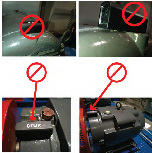
Figure 6.3 Examples of places you should not mount sensors.
