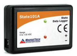
The State 101A data logger monitors and records the occurrence, duration and status of predetermined events by measuring changes in voltage. Typically connected to a relay or switch, this data logger features a removable screw terminal block to easily disconnect and retrieve the logger for data download without disrupting wiring connectivity.
