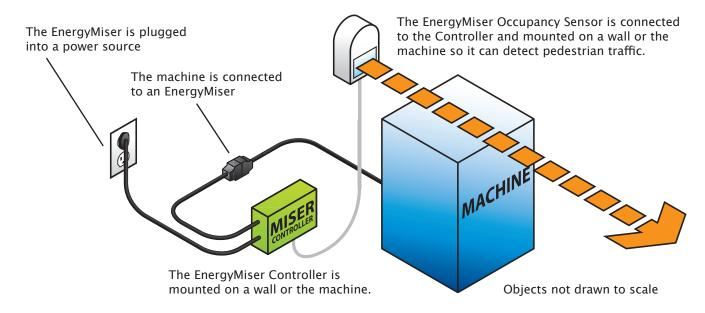
Internal EnergyMisers use sales based intelligence to power down the cooling system while leaving lighting and controller electronics on. While the cooling system is powered down, the internal EnergyMiser monitors the room's temperature and automatically re-powers the cooling system at regular intervals to keep the product cold. Internal controllers are best suited for high traffic areas.
