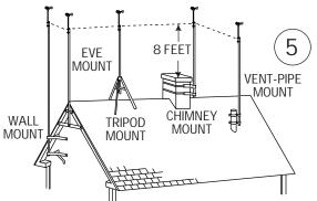
Follow the instructions supplied with the antenna mount and secure the mast to the mount.
