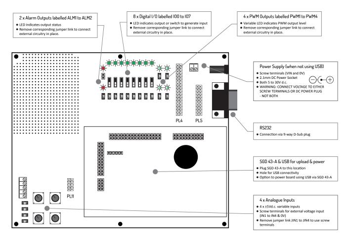
The main connection is that of the SGD 43-A supplied as part of the SGD 43-A-DK+ development kit. The board can be powered directly by connecting a USB cable to the rear of the display. Whilst connected the USB will provide power to both the display and the development board.
