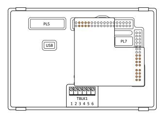
The diagram (above-right) indicates the pins on the SGD 43-A that the S43-TP should be connected to.
