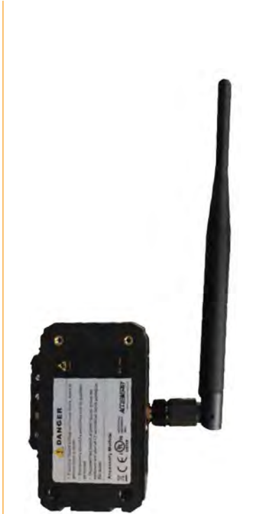
AXM-MESH transceiver module that can only be attached to the Acuvim II series meters.
