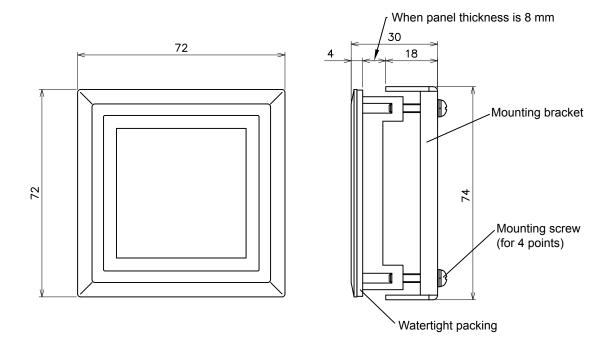
How to install PXF4 with the adapter
