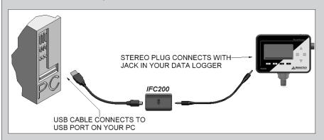
Insert the USB connector of the IFC200 into an available USB port. Fully insert male connector of the IFC200 interface cable into the female receptacle of the data logger\*.
