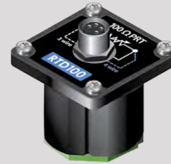
M8 connector cable or terminal block. Works with 2-, 3-, 4-wire RTDs.
