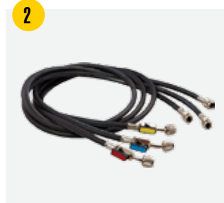
Premium 3-Pack 5' Hoses (Varies by kit. See chart below) • 1/4" SAE 45° fittings • 800Psi working pressure • 4000Psi burst pressure
