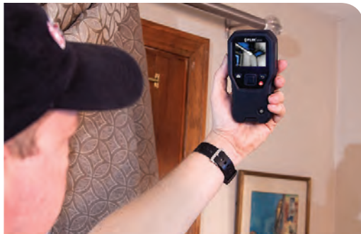
Scanning ceiling & wall joint for moisture issues
