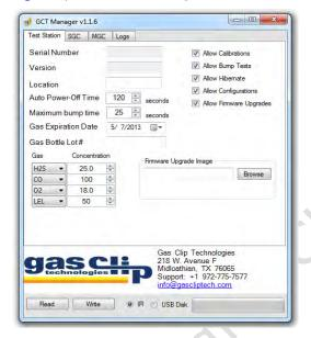
The GCT Manager software can communicate with the Clip Dock through IR or USB as selected by the radio buttons. IR communication is handled through Bay 1 of the Clip Dock and if the IR Link is placed into Bay 1. For IR communication, connect the Clip Dock to a charger and place the GCT IR Link into Bay 1. Direct USB operation with the memory stick connected to the PC offers faster transfers or configuration without a GCT IR Link.
