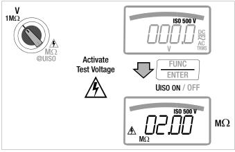
Auto-ranging is active during insulation resistance measurement.
