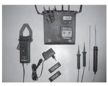
Clamp-on ammeter MZ 1005 Art. no. Z209C for current measurements of 0,1 - 1000 A only in Ex – I areas. Power supply unit NG64 Art. no. Z209P for charging the accumulator NiMH accumulator EXM-AK9/T4 Art. no. Z209A Lithium battery EXM-LB3 Li/T6 Art. no. Z209B Temperature transmitter TMZ 25 Art. no. Z209T between - 80 and + 600 °C in Ex-I and Ex-II areas universal sensor EXM-TFU Art. no. Z209U surface sensor EXM-TFO Art. no. Z209S
