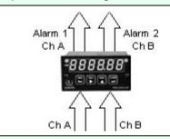
A single Laureate dual-channel counter will handle two repetitive fill operations by counting from zero up to a preset, or down from a preset to zero. A dual setpoint relay board is required.
