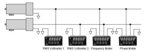
Synchronization of two motor generators requires that the voltage outputs of the generators be close to each other, that the two frequencies be identical, and that the voltage waveshapes be in phase.
