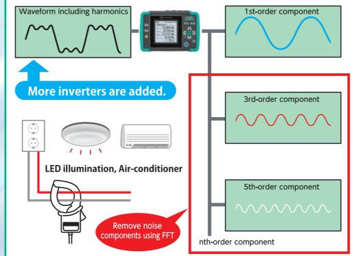
Unlike to traditional Ior measuring apparatus, less susceptible to harmonics noises.
