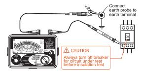
Check the circuit under test is not energized as follows.
