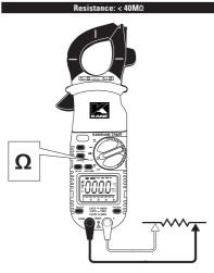
Do not measure resistance on a live circuit.
