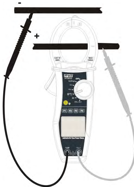
Fig. 11: DC power measurement
