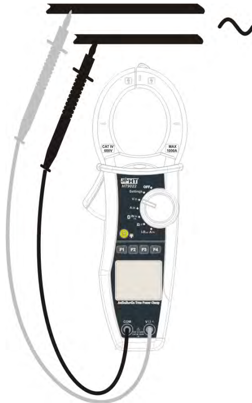
Fig. 6: AC+DC voltage measurement
