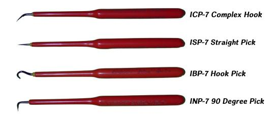
Each hook and pick is made of high carbon polished steel in a permanently attached aluminum handle which is then double-insulated; tested to 10,000 Volts AC and rated for 1000 VAC / 1500 VDC protection.
