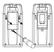
Replacement should take place in a non-hazardous area using a 9V Ni-MH rechargeable battery.
