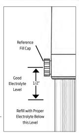
Always use the appropriate fill solution for your pH electrode. Typically, single junction pH electrodes use the <u>HI7071</u> electrolyte solution (3.5M KCl + AgCl), while double junction pH electrodes use <u>HI7082</u> electrolyte solution (3.5M KCl).
