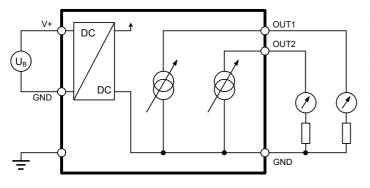
The maximum permissible cable length, connecting the unit to other devices, is determined by the total resistance resulting from the addition of the cable resistance and that of the devices connected in series with the unit. This resistance should not exceed 500  $\Omega$ .
