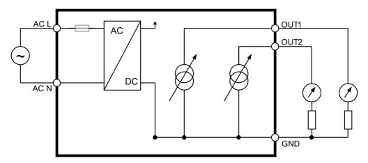
The maximum permissible cable length, connecting the unit to other devices, is determined by the total resistance (cable resistance + devices connected in series with the unit). This resistance should not exceed 500  $\Omega$ .
