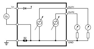
Terminal block diagram (analog outputs only)
