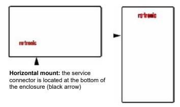
**Vertical mount:** the service connector is located either on the left side or on the right side of the enclosure.
