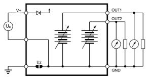
Electrical diagram for current outputs
