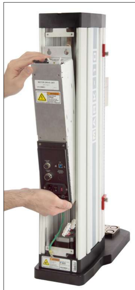
Removing the MDU
