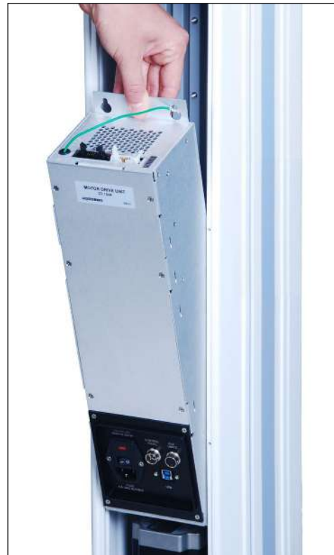
Removing the MDU
