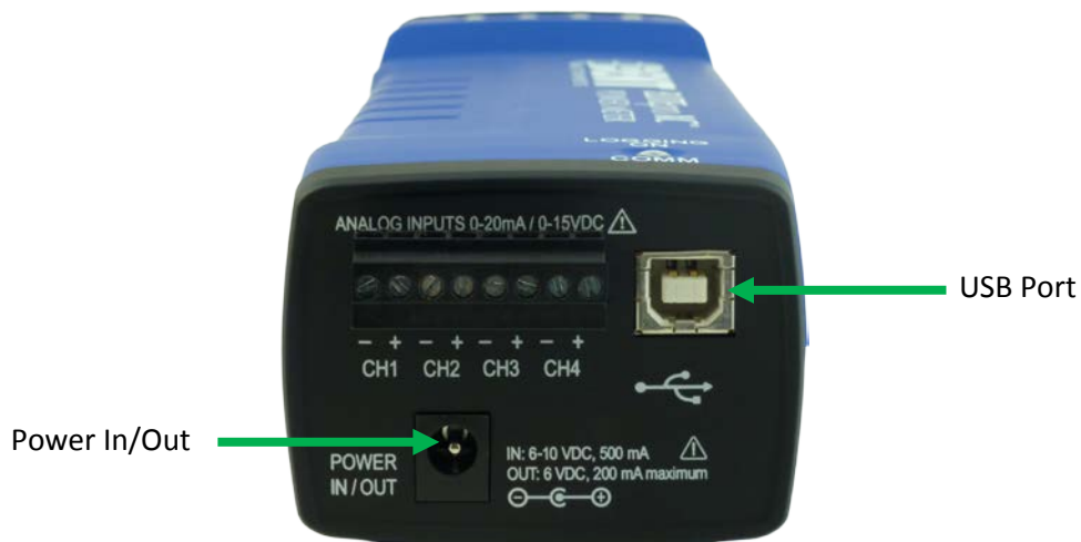
Power End Panel Connections
