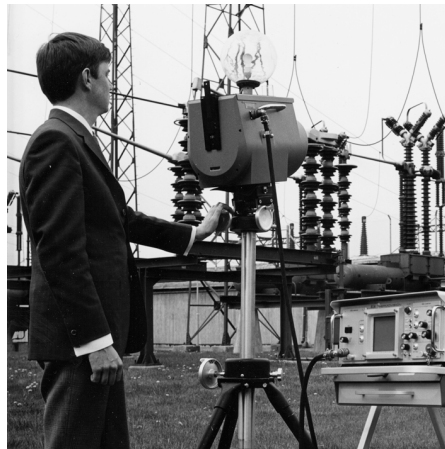
Figure 13.2 1969: Thermovision Model 661. The camera weighed approximately 25 kg (55 lb.), the oscilloscope 20 kg (44 lb.), and the tripod 15 kg (33 lb.). The operator also needed a 220 VAC generator set, and a 10 L (2.6 US gallon) jar with liquid nitrogen. To the left of the oscilloscope the Polaroid attachment (6 kg/13 lb.) can be seen.
