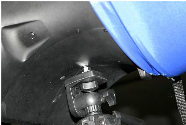
Figure 27: Mount Hood Base to Telescopic Stand
