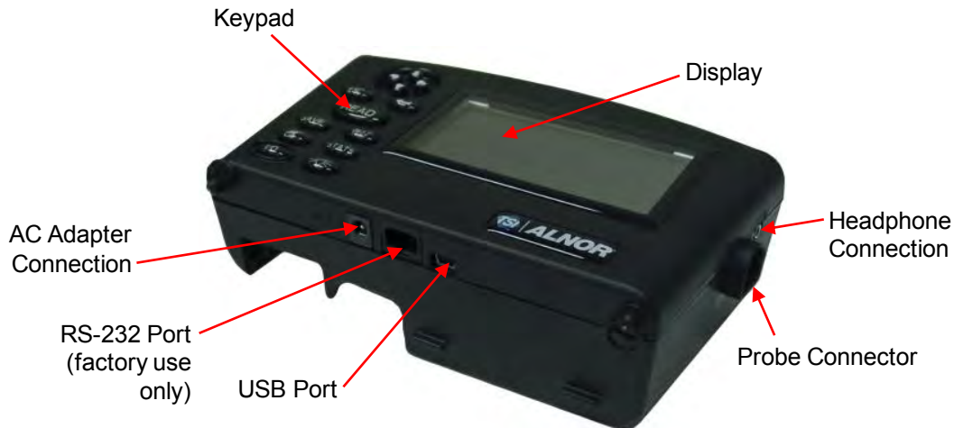
Figure 1: Features of the EBT730/EBT731 Micromanometer, Front View
