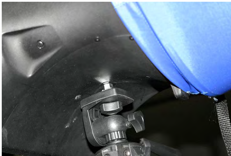
Figure 27: Mount Hood Base to Telescopic Stand
