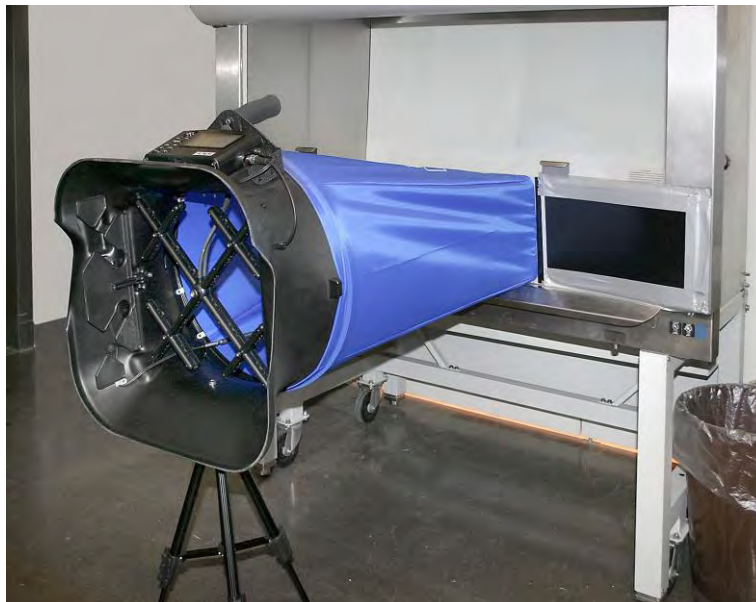
Figure 23: Direct Inflow Measurement Hood
