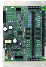
36/72-ch Bottom Feed Configuration Panel 1
