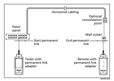
Figure 3. Permanent Link Connections for Links Up to Cat 7<sub>A</sub>
