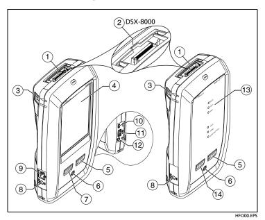
Figure 1. Connectors, Keys, and LEDs (Versiv 2 shown)
