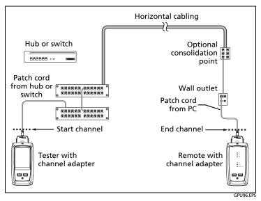
Figure 4. Channel Connections for Links Up to Cat 7<sub>A</sub>
