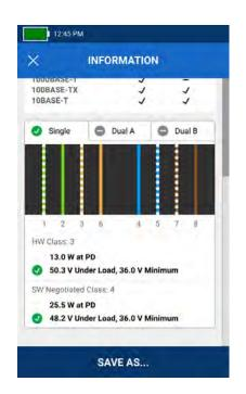
The LinkIQ<sup>™</sup> screen with network speed and PoE Power Sourcing Equipment (PSE) diagnostics including result of PoE loaded test.
