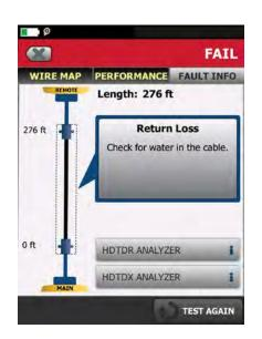
DSX CableAnalyzers<sup>TM</sup> provide the most advanced diagnostics for troubleshooting difficult cabling problems.
