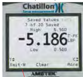
Gauge will transmit result WITH units.
