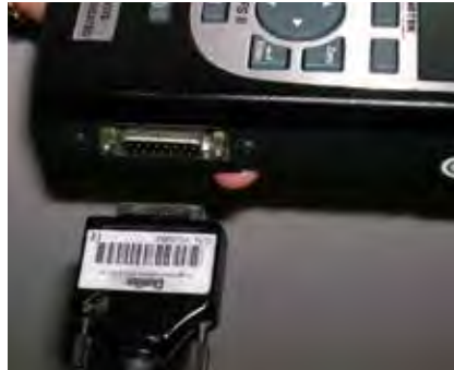
Carefully mate the connector on the SLC or STS sensor to the connector on the side of the DFS II-R-ND gauge.
