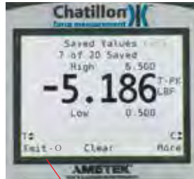
Gauge will transmit result WITHOUT units.
