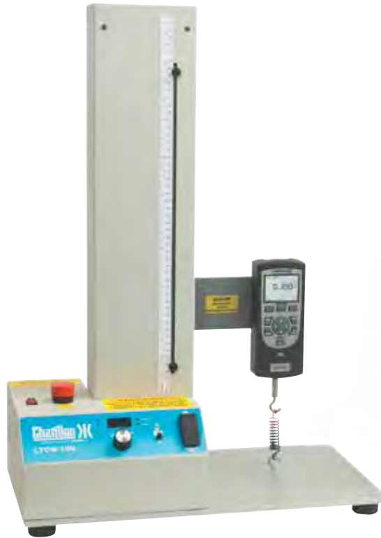
Shown: DFS II digital force gauge mounted on the LTCM-100 motorized tester.
