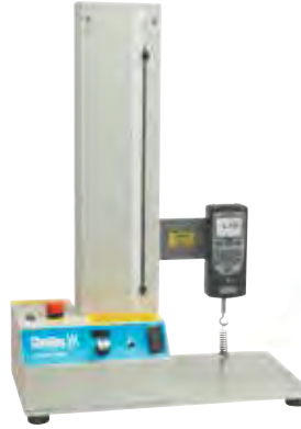
DFS II gauge mounted to LTCM100 tester
